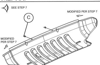
RAISE SPLASH SHIELD BEHIND BUMPER AND ALIGN HOLES TO INSERT CENTER TWO (2) BOLTS INTO U-NUTS.
