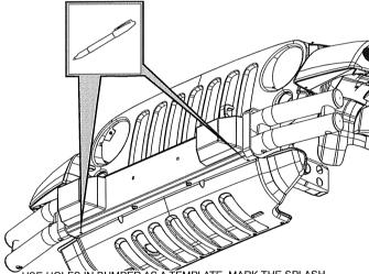
USE HOLES IN BUMPER AS A TEMPLATE. MARK THE SPLASH SHIELD TO LOCATE OUTER HOLES. REMOVE SPLASH SHIELD AND DRILL 7/16" DIAMETER HOLES.
