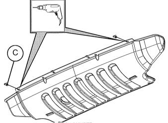
DO NOT DRILL THRÔUGH BUMPER. INSTALL TWO (2) U-NUTS.
