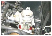
**5.** Install one gasket (#4) on the intake manifold, then the Poweraid spacer (#1), with the other gasket (#4) on top of it. Next install the throttle body using the four provided 6mmx50mm bolts (#2) and washers (#3), and tighten to manufacture's specifications.
