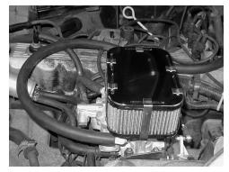
Carburetor Mounted with Air Cleaner Picture 10
