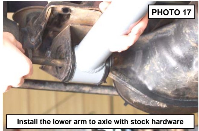
Install the lower control arms with 9/16" x 4" bolts
