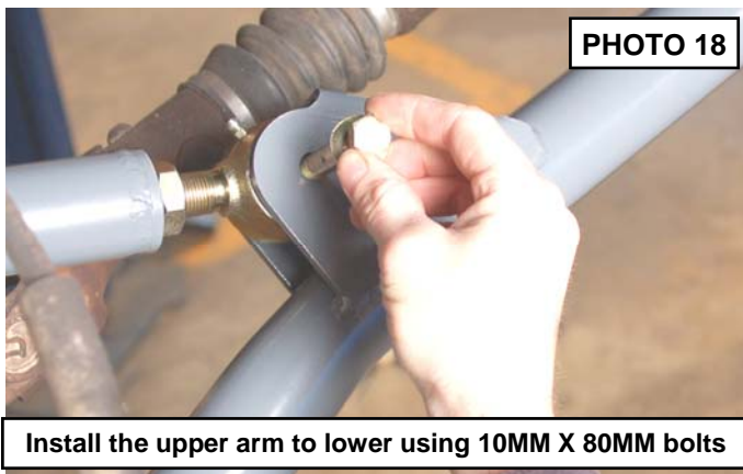
Install upper arm to axle with 10mm x 80mm bolts
