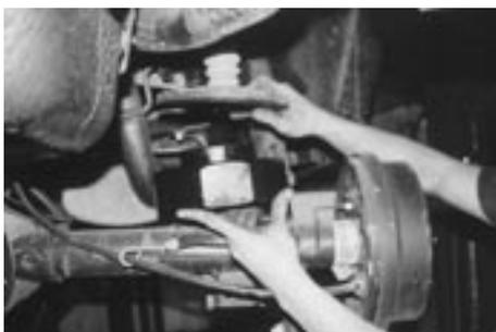
29. Install the factory spring above the spacer. A spring compressor will make this installation much safer and easier.
