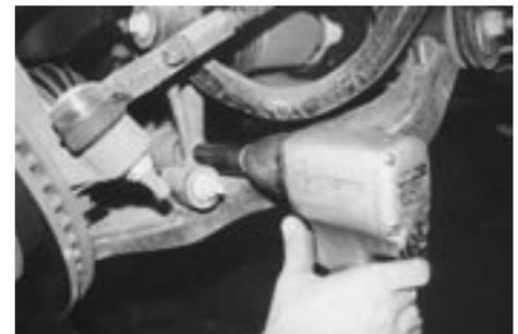
22. A jack stand is a convenient way to raise the knuckle into position so that the upper A-arm can be connected to the knuckle. Torque to factory specifications.
