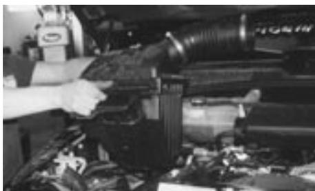
4. Pull the air filter assembly from the vehicle and set aside.
