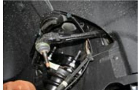
*Note: If necessary remove lower A arm bolts to allow more droop.*
