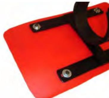
**Step (2)** Press license plate holder over the the front tube bumper as shown.Center license plate holder and secure it in place with (1) 1/4" x 1 1/2", (1) 1/4" flat washer, and (1) 1/4" nut.
