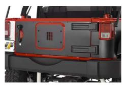
**IMPORTANT:** Warrior only recommends one method of installation. This method includes drilling holes and pop-riveting the tailgate cover into place, and will be the method covered in these instructions. Actual mounting hardware & method are at the discretion of the installer. Any gasket or sealants used are also at the same discretion. All covers are designed to overlay the existing factory tailgate with factory hinges and latches.
