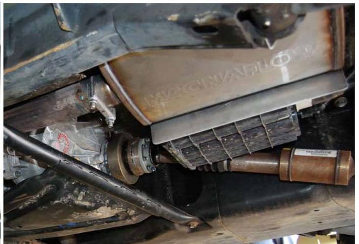
6. The above picture shows the location of where the muffler will mount. Hold the muffler up into its location, and mark the pipe at the ends of the muffler with a felt tip marker. Keep in mind that the pipe will need to be longer than where you marked so that the muffler can slide onto the ends of the pipe. The sleeve on the end of the muffler should be about 2", but measure yours just to be accurate. Take that measurement and mark exactly where you'll be cutting on the pipe.
