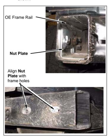
b. Position kit bumper on vehicle. Secure bumper to frame rail on both sides using kit, 10m-1.5x40 bolts & washers, for forward two holes and kit 1/2" x 1-1/2" bolts & 1/2" washers through nut plate inside frame rail. Do not tighten at this time.
