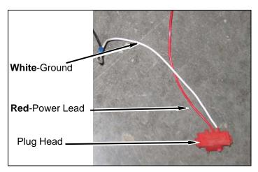
b. Prepare frame for ground wires by removing a small section of paint to provide a good ground to harness. Use kit self tapping screw to ground the white wire on plug. (Note: Be sure that plug harness locations are near the inside of frame rails to give them enough slack to reach the light pockets once installed.).
