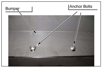
**d.** Insure bumper is centered and level. Tighten down all hardware at this time.
