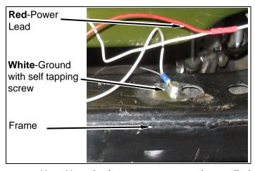
c. Use kit red-crimp connector and supplied wire to extend and connect both red positive leads to each other with plenty of slack in the harness to reach upper passenger side factory tail light harness underneath carpet near roll bar.
