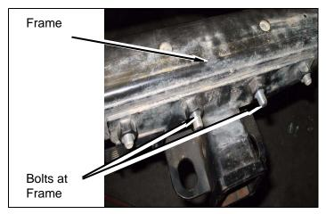
b. Install kit anchor bracket with two kit flange nuts (12m-1.5). Center kit anchor bracket flush with the mounting surface and tighten down kit flange nuts..
