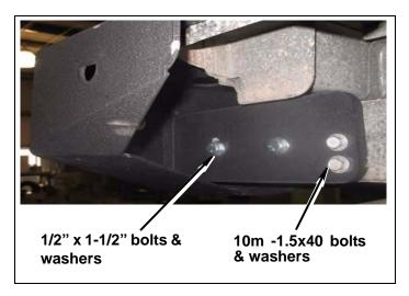
**c.** Install two *kit* **bolts** (3/8-16x1) through bumper center plate and into *kit* **anchor bracket**..
