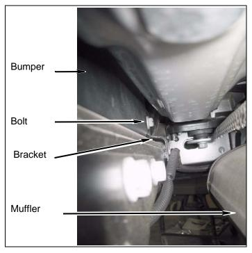
**b.** Remove two bolts from each bumper bracket at frame and remove bumper.
