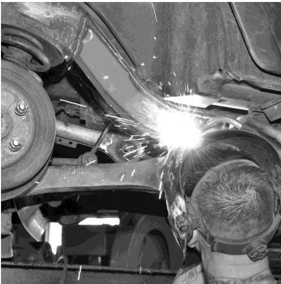
Picture 4, Tack in place
