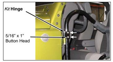
a. Install kit mirror mount onto driver rock door using both 5/16" button head bolts that were previously removed from hinge. (Note: Kit mirror mounts are offset for both Dvr & Psg sides; be sure that the slots are off set toward the front of the hinge.).
