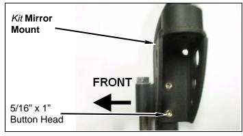
**b.** Install O.E. mirror onto *kit* **mirror mount** using *kit* **bolt** (**8M-1.25 x 20**) & **washer**.
