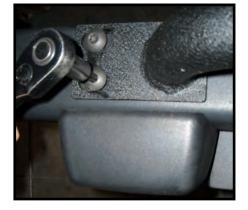
3. To use factory tow hooks with this light bar, place tow hooks on top of Light Bar mounting plates. Be sure to use the correct tow hook for each side of the vehicle. Tighten Light Bar into place using factory torx head bolts.
