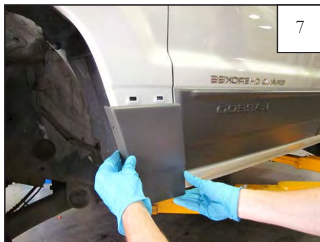
Pull firmly to remove upper factory fasteners in front side cladding piece from fender. Clean exposed sheet metal.
