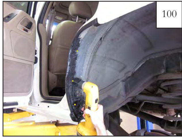
100 Remove part and drill marked locations using a 3/32" drill bit (4 locations).
