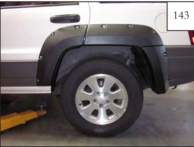
Completed rear flare installation.
