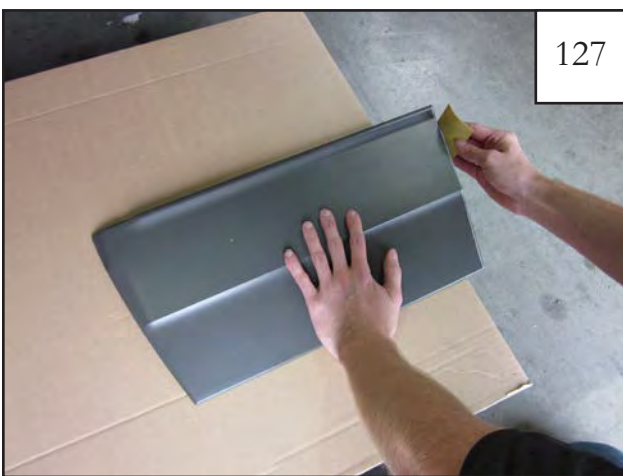
Using sand paper, smooth cut edge of the factory side cladding.
