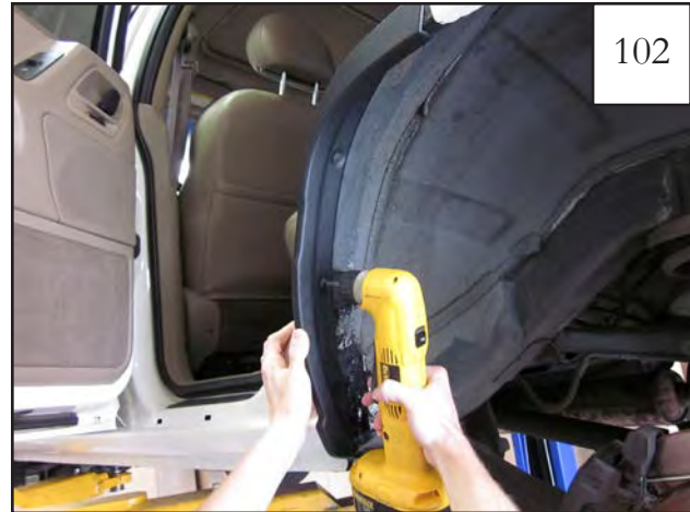
102 Place cover piece back on vehicle. Using a #2 phillips head, install screws (SW1-0056) through cover piece into holes drilled in step 100. Remove excess caulking along edges if needed. Tip: A power drill works best, do not overtighten.
