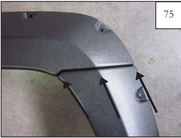
75 Check alignment of main flare and bumper piece to each other. Line up the three style lines.
