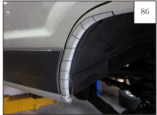
Mark vehicle for cutting: Make marks from inner wheel well to line drawn in previous steps about 2" apart as shown in picture. Make marks closer together around tight corners and style lines.
