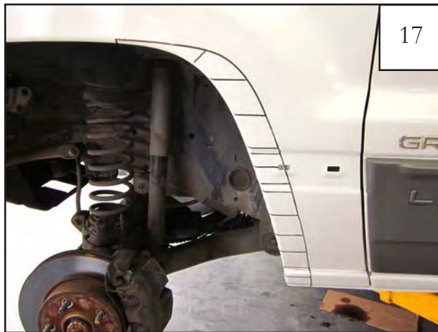
17 Mark vehicle for cutting: Make horizontal marks from wheel well to line drawn in previous steps about two inches apart as shown in picture. Make marks closer together around tight corners and style lines.
