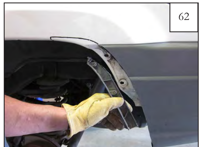
Remove trimmed bumper support bracket.
