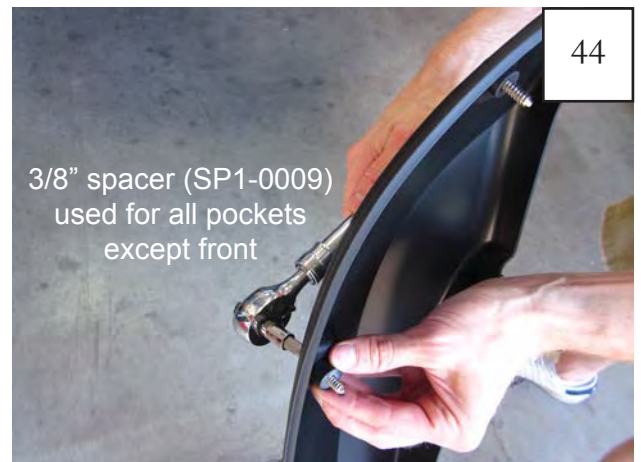
For all remaining pockets, install a #45 Torx screw (SW1-0045) through pocket hole and secure with rubber spacer ( SP1-0009 ) using supplied #45 Torx bit (SW1-0052). Drive screw into spacer until tight. Repeat for all remaining pockets.
