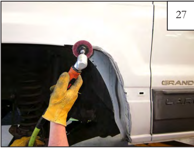
Using an angle grinder or sandpaper, sand the chipped paint along bent edge of the wheel well.
