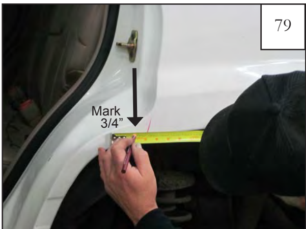
79 Measure 3/4" toward the front of the vehicle from the mark made in previous step along fender lip. Using a grease pencil, make a mark.
