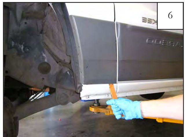
Using a pry tool, separate the factory front side cladding from the sheet metal along the bottom taped edge.
