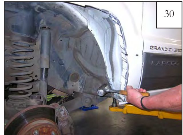
Using a hammer, pound the tabs made in the inner pinch weld flat against wheel well.
