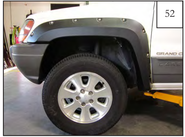
Completed front flare installation.
