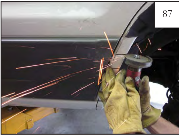
Using a cut off wheel, sawsall or other suitable tool, cut along horizontal marks from wheel well to vertical line. NOTE: DO NOT OVERCUT!
