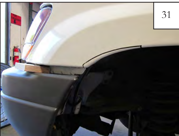
Use a small wood block to prop the bumper away from the fender in preparation for sheet metal trimming.
