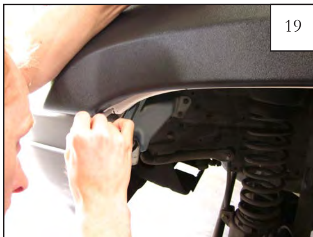
19 Hold the flare up to the fender as a guide. Make a mark connecting the two marks made in step 18.
