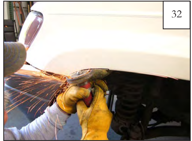
Starting at the front edge, cut out mark shown in Step 20.
