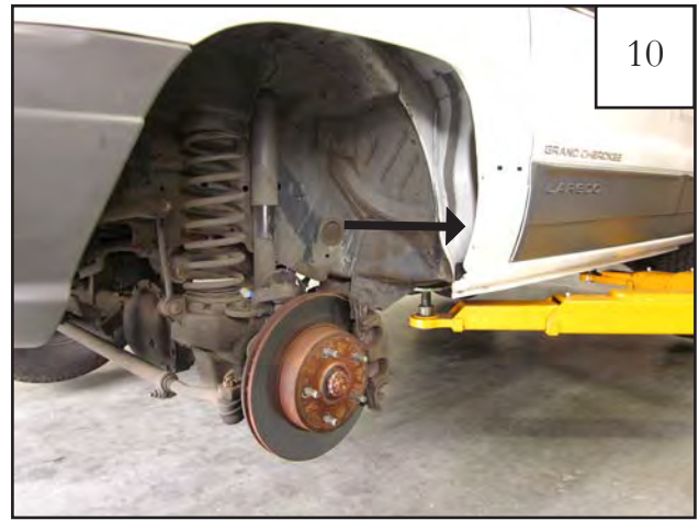
Remove splash shield and push sound dampening foam back into inner wheel well behind the fender. NOTE: If debris is present in inner wheel well, remove before continuing installation.
