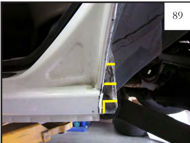
Mark vehicle for cutting: Make horizontal marks on the inner pinch weld flange approximately 1-1/2" apart.
