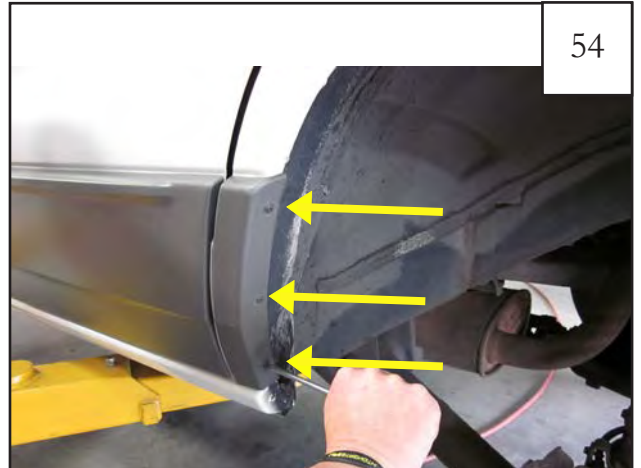
Using a #2 Phillips Screwdriver, remove factory screws from upper side cladding (3 places). Remove cladding.
