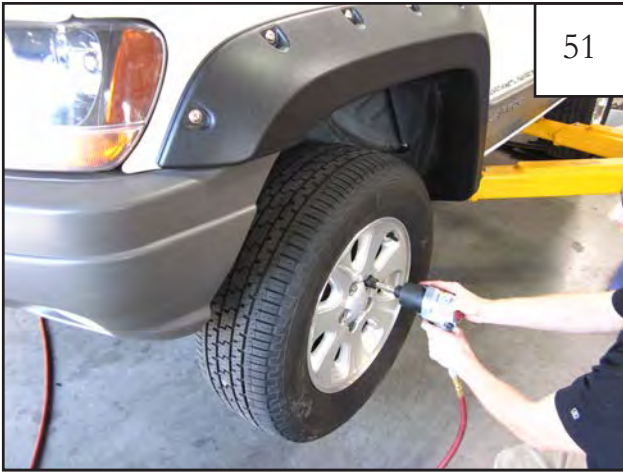
Re-install tire using an impact wrench.
