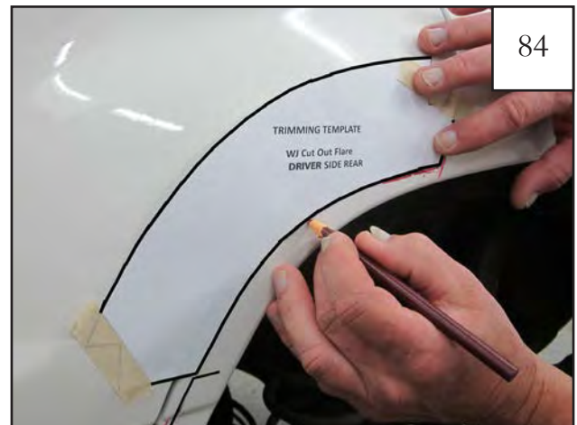
Using a grease pencil, draw a line along the lower edge of the template to connect marks made in previous steps.
