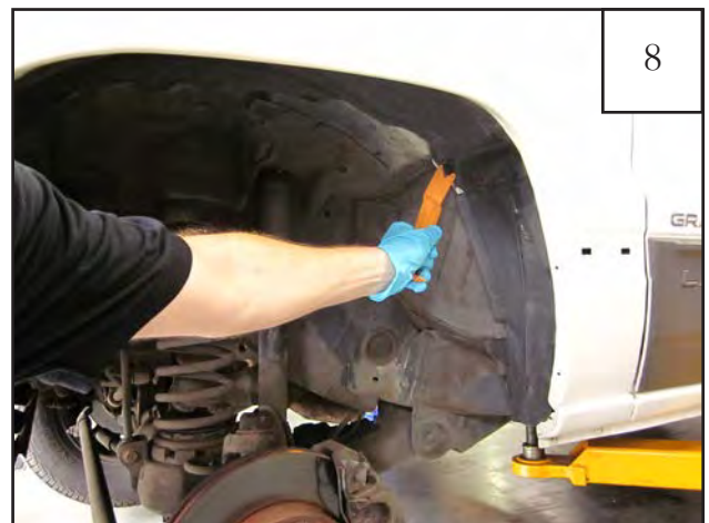
Using a pry tool or utility knife, remove factory fasteners from wheel well splash shield (9 places).
