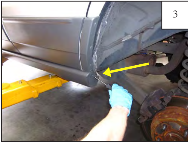
(Note: For models with Rocker Panels installed) Using a #2 Phillips Screwdriver, remove screw from rocker panel in rear wheel well.
