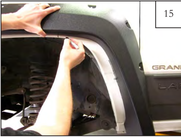
15 Hold the flare up to the fender as a guide. Make a line connecting the marks made in steps 13 & 14.
