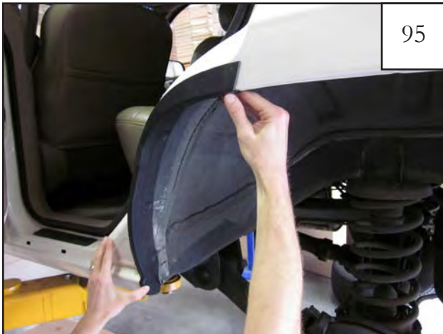
Hold cut cover piece in place on vehicle. Confirm fit to cut areas and make adjustments as needed. Parts are marked on the inside. Driver's side: D2 for cut cover piece.
