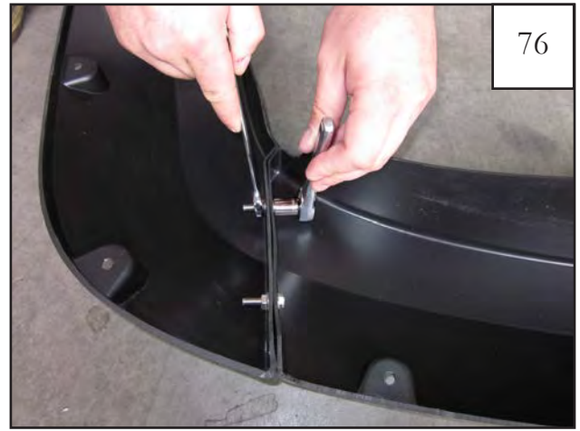
76 Once satisfied with alignment, tighten all screws.
