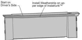
Make sure that Instatrunk<sup>™</sup> Assembly is level.
