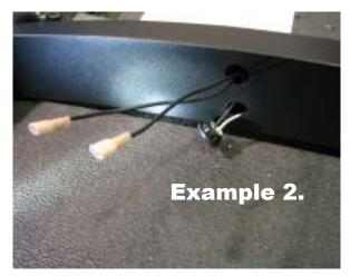
Step 2. Feed supplied black wire up through Bull Bar and out the bigger front hole. Pull the black LED wire out the top hole as well. Attach female connectors to both black wires. (Example 2.)
