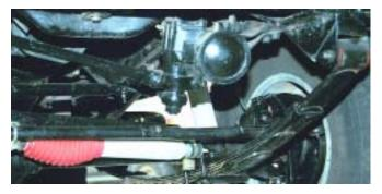
**Step 1** Remove the bolt from the coupler that couples the intermediate shaft to the input shaft of the steering gearbox.
