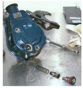
**Step 6** Grip the pump by its drive shaft and surrounding case, then use a soft-faced mallet and tap around the edge of the tin reservoir to remove it from the pump.
