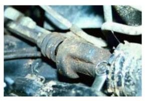
Step 2 Remove the power steering hoses from the steering gearbox.
