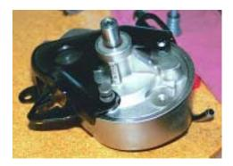
**Step 10** Install the pump pulley onto the pump. Always use a pump pulley installer to push the pulley back onto the pump drive shaft. The hub of the pulley should be flush with the end of the drive shaft.
