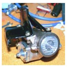
**Step 2** Connect the intermediate shaft coupler to the input shaft of the gearbox.
