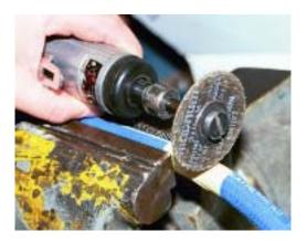
Step 10 After the hose has been cut to length, clean out the hose to remove any debris.
