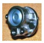
Inspect the new pump to make certain it is the proper one for your application. Although all P-type pumps look very similar, there are distinct differences. All 1980 and newer Saginaw equipped vehicles were equipped with metric pumps and an o-ring type pressure fitting. 1979 and earlier vehicles were equipped with SAE pumps containing a flare type fitting.
