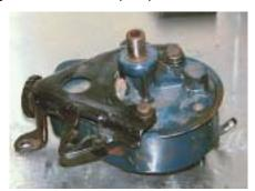
**Step 3** Remove the bolts or stud bolts from the back of the pump. In most applications there are two, but some only have one.
