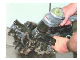
Step 7 Using a pitman arm puller, remove the pitman arm.
