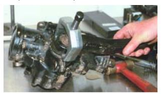
Step 8 Remove the mount bolts that retain the gearbox in the chassis. On some vehicles you must remove the steering gearbox with the mount brackets attached and then remove the mount brackets once the gearbox is on the workbench. As you are removing the gearbox, you can then disconnect the intermediate shaft coupler from the input shaft of the gearbox. You might have to use a mallet and tap on the coupler to get it to slide off of the input shaft.
