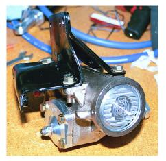
Step 2 Connect the intermediate shaft coupler to the input shaft of the gearbox.
