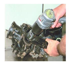
Step 7 Using a pitman arm puller, remove the pitman arm.
