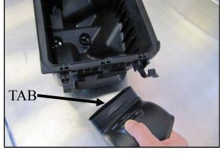
**5.** Depress the locking tabs holding the factory air scoop in the lower half of the airbox and remove it.
