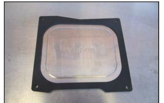
17. Mount the self adhesive Gasket (#7) onto the underside of the Air Box Lid (#6) and peel off the protective film on the top. Mount the lid onto the Air Box using four remaining 1/4-20 x 1/2" Button Head Bolts (#10), and 1/4" Flat washers (#12).
