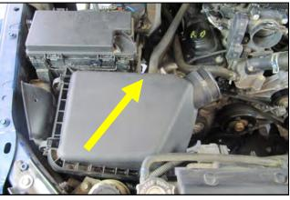
**3.** Disconnect the crankcase breather line fromt the top of the airbox. Remove the entire airbox as an assembly by unseating it from the mounting grommets in the inner fender and lifting upward.
