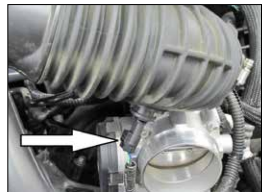
6. Lift up the intake tube, disconnect the inlet air temperature electrical connection then remove the intake tube from the vehicle.
