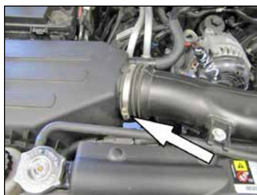
4. Loosen the hose clamp securing the factory intake tube to the air filter housing.
