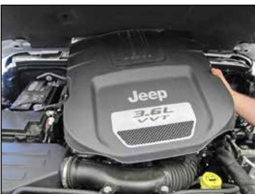
2. Lift up and remove the engine cover.
