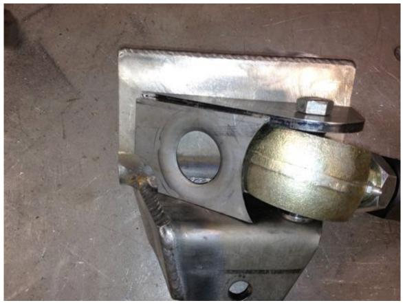
15. Reinstall and tack weld the control arm brackets on the frame. Double check the front to back location and make sure they are the same side to side.
