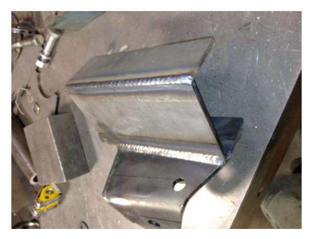
14. Decide which side you want the upper control arm on. It usually goes on the side that the drive shaft is on. Driver side for a TJ or YJ. Weld the upper control arm top plate and gusset as shown below. There of two of these brackets included, you can use both and make a triangulated 4-link. The opposite side frame bracket without the upper control arm gets the 2 vertical gussets.
