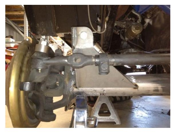
29. Determine the mounting location for the frame mount track bar bracket. The track bar needs to be parallel to the drag link so you may need to trim the bracket to mount higher if needed. Tack weld the bracket to the frame.
