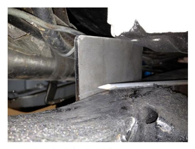
11. Remove the control arm bracket and cut at the line.
