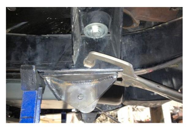
10. Mark the bracket where the top edge of the frame is.
