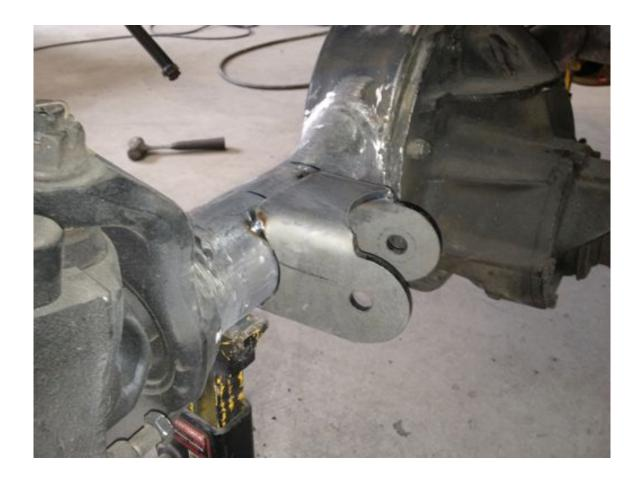
19. Mock up the single upper control arm mount (may require fabrication or purchase of an axle bridge for over the diff housing). Do not weld entirely to a cast diff housing, it will not hold. The side to side location is usually pretty tight so you may want to wait until you place the axle back in the vehicle to finalize this mount.
