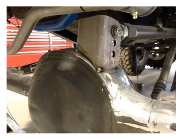
27. Measure center to center of the upper control arm bracket, cut and tack weld the tube for the upper control arm and install in the vehicle.
