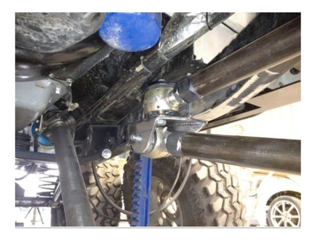
26. You may want to raise the front axle up to where you think full bump is to check clearance for the upper control arm. Once you have determined a upper control arm side to side location you can fabricate the upper control arm bracket.
