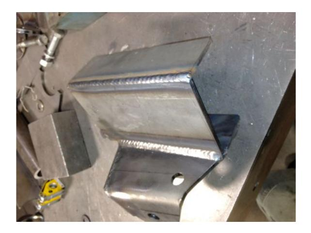
14. Reinstall and tack weld the control arm brackets on the frame. Double check the front to back location and make sure they are the same side to side.
