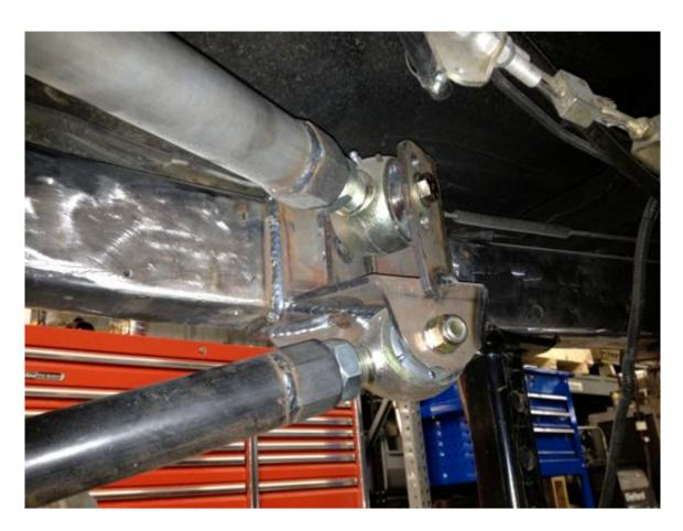
10. Mark the bracket where the top edge of the frame is.
