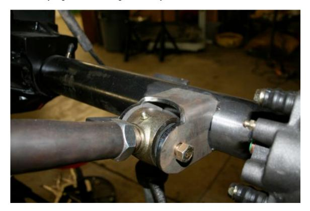
18. Mount the axle truss with the upper control arm brackets. This is typically mounted with the top level. Tack weld to the axle tube
