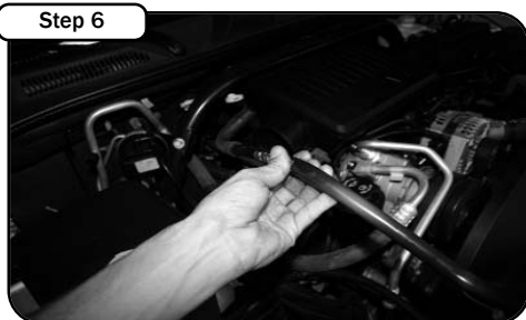
Remove the vent hose from Commander models. Remove hose to tee junction on Grand Cherokee models.
