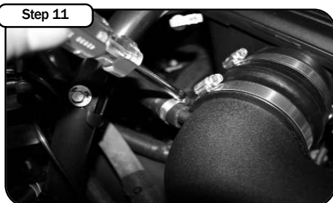
Tighten clamps on intake tube to plenum box with 5/16 nut driver. Place new vent hose onto tube and tighten clamp using 1/4" nut driver. (on Grand Cherokee models the excess vent hose will need to be trimmed to length approx. 4")
