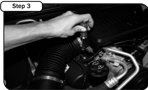
With 5/16" nut driver loosen top of OE intake tube.
