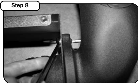
With screws, nuts, and washers provided, place new aFe tube onto housing and tighten using a phillips screwdriver and 7/16" socket or wrench.
