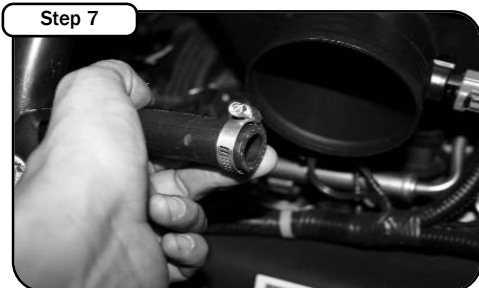
With 5/8" hose provided, install new hose into valve cover vent (on Grand Cherokee models connect hose to vent tee). Place mini clamp onto hose and wait to tighten on new intake tube.
