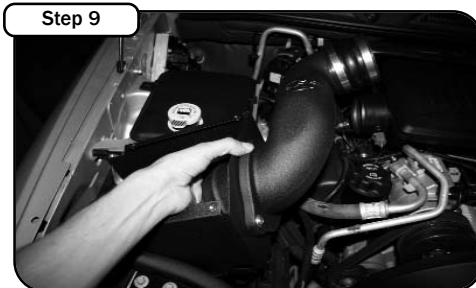
Place the hump coupler onto the tube with clamps provided and install intake into vehicle.
