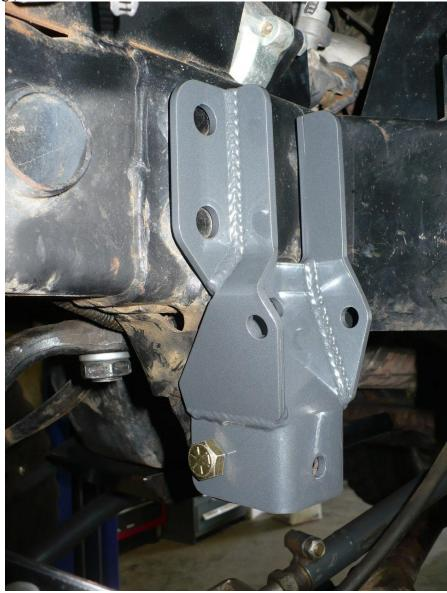
5) Install the 2 7/16" bolts with washers under both the bolt and under the top locks. Note, lower bolt must be installed with nut on outside of brkt to clear TB. Upper bolt orientation is up to the installer but advice to install in the same orientation as lower with the nut on outside of bracket.
