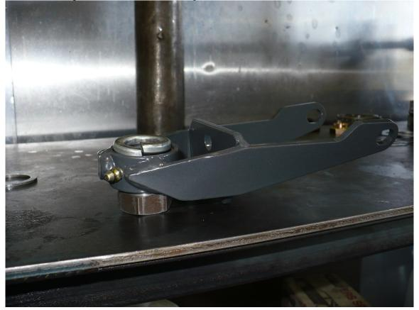
13) Next, slide the whole assembly into place over the 8069-01 Track Bar Brace and start the pitman arm stud. Tighten finger tight.
