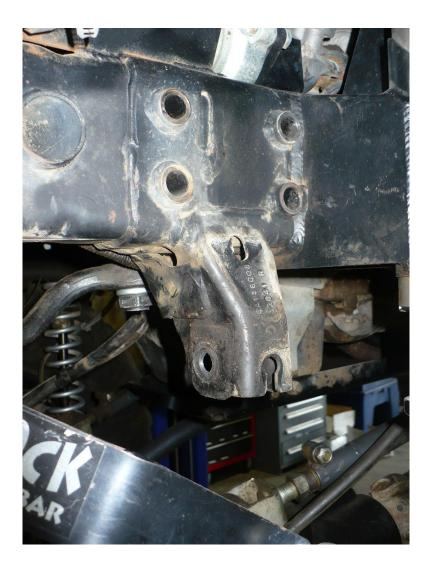
4) Next, install the PPM-8069 Track Bar Brace by fitting it over the factory track bar mount and installing the 9/16-12 UNC bolt provided in the kit. (Note: do not install the nut at this time, the bolt is just to hold the bracket in place for the time being.)
