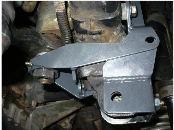
14) Next, align the outer bolt holes so the 7/16-14 x 1.0" long bolts provided in the kit can be installed. An alignment bar or screw driver will be helpful in pulling the mount into the proper location.
