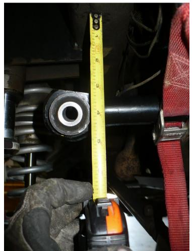
Bump stop measurement shown from bottom of frame to mounting hole with stock Track Bar.
