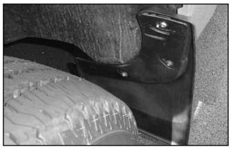
After tightening the QuickTurn<sup>™</sup> fastener, tighten the (2) hex head screws while pressing the MudFlap against the fender. For passenger side, turn front wheels fully to the right and repeat steps 1-9.
