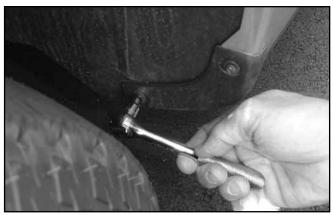
Using the appropriate socket or nut driver, remove these fasteners. They will be reused later.
