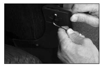
While pressing the MudFlap against the fender for a tight fit, tighten the QuickTurn™ fastener with the hex key. Make sure the indicator moves to the locked position and then continue tightening until snug.
