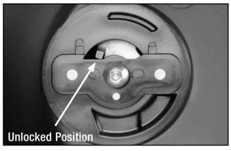
Locate the QuickTurn<sup>™</sup> fastener on the MudFlap. Ensure that the QuickTurn<sup>™</sup> fastener is in the fully unlocked position using the hex key provided.
