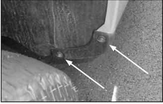
Locate the fasteners holding the plastic fender guard to the fender.
