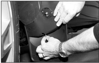
Using the supplied bolt and washer, position the MudFlap against the contour of the fender flare, and put the bolt through the opening in the MudFlap and then through the hole where the plastic rivet was. Place the supplied nut on the bolt threads. Do not tighten at this time.
