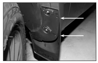
Optionally, the (2) screws (with washers) can be used in the indicated holes (holes 1/8" will have to be drilled in the plastic flare, no metal will be contacted).
