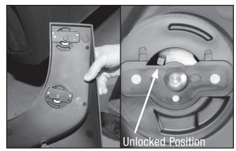
Using the MudFlap marked "LH", ensure the QuickTurn™ fasteners are in the unlocked position.
