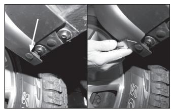
Start the installation by locating the plastic rivet indicated. The rivet head will need to be cutoff and removed (also remove the inner portion, you can reach around for access).
