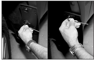
While pressing the MudFlap against the fender contour, rotate the QuickTurn<sup>™</sup> fastener with the supplied hex key. The fastener will rotate to the "lock" position and stop. Continue turning to tighten the flap onto the flare. Repeat for the other QuickTurn<sup>™</sup> fastener.
