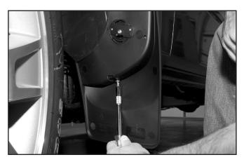
The lower screw/bolt can now be tightened (nut on back may need to be held with a wrench).
