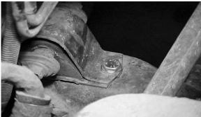
**Step 3:** From under the hood remove the motor mount bolt on the driver's side.(Shown above on the left.) Then replace it with the new M10-1.50 x 35mm bolt and flat washer supplied.(Shown above on the right.) Once this bolt is tightened you are done under the hood.
