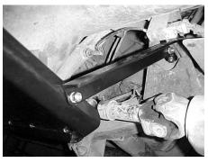
**Step 9:** Take the strut rod and attach it between the mounting bracket installed in Step 4 and the skid plate using two 3/8-16 x 1" hex head bolts, lock washers, and hex nuts. The end with the square cut is the bottom of the strut rod. This gives you the most clearance for the differential and driveshaft.
