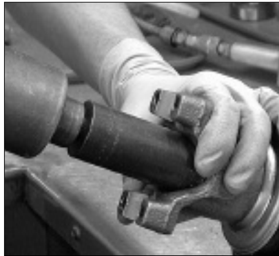
1/2" impact gun on pinion nut
