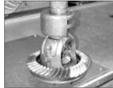
Carrier bearing puller
