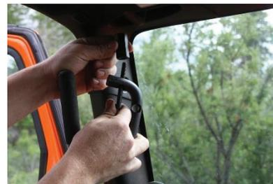
Install the short 8mm bolt through the top hole of the handle, then through the short spacer. Insert the bolt with the handle and spacer into the upper hole of the windshield frame (adding oil to both bolts) **(Do not tighten! Only turn it in a couple of threads).**
