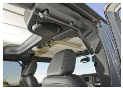
using a 5mm hex wrench, tighten both bolts to 120 in-lbs of torque.
