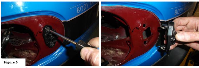
4. To prepare the wiring for the lights, the 5-wire to 4-wire converter must be installed. As mentioned above, it is your responsibility to choose which method you prefer for your wire connections and splices. To install the converter, you should remove the lower plastic threshold below the rear gate by removing the (5) Philips head screws, then gently pulling upward on the plastic trim starting at one end. This is where you can run wires across the vehicle. See **Figure 7.**
