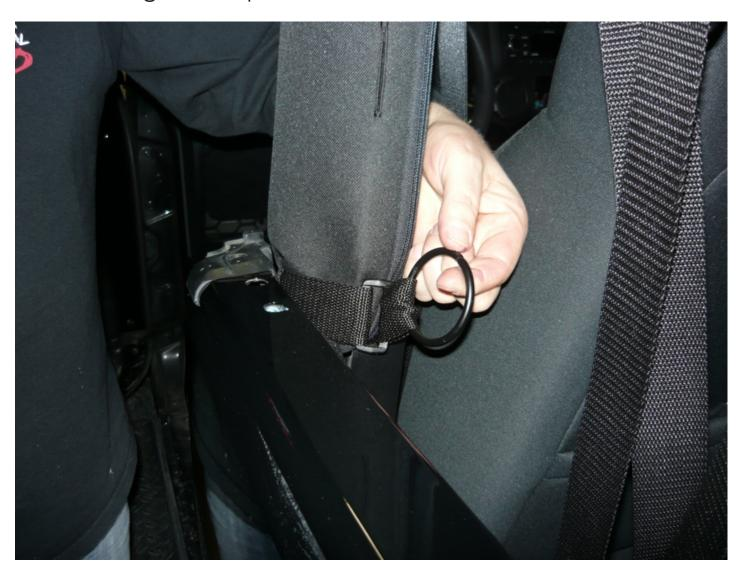
The straps can now be installed and tighten in the order shown in the photo. Straps 1 and 2 are installed first and pulled evenly and tight. Follow next with 3-6 in order. Strap 5 has to be adjusted at the top as well. After all 6 are installed go through and adjust each one till the side looks uniform. Strap number 7 can now be installed. Both sides need to be attached. The back side uses the loop from the strap that
