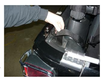
You will first install the back section. Using the position of the dirty dog tag to orient top from bottom. This tag should be readable from the outside. The bottom 4 straps will need male buckles installed on each side. See back page. The bottom male buckle will connect to the straps you have just installed.
