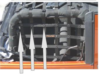
You can now skip the next two straps and go to the final straps at the front corners. These straps wrap over the speaker bar. Wrap the long strap around over the front of the speaker/roll bar and bring under and around up the side and feed into the ladderloc. There will be two ladderlocs. The second one is used for the side strap. See photos next page
