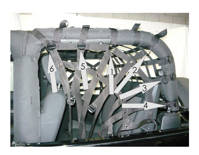
Find the strap that has a metal ring and a plastic loop installed on one end and velcro sewn to the other end. This strap is installed on the roll bar beside the seat. The strap wraps around the roll bar passes through the plastic loop and the velcro hooks onto itself. Be sure that the strap gets pushed below the body side so it falls below the padding of the roll bar. The ring should pull out toward the back.
