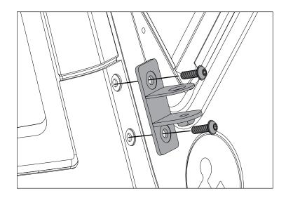
3. Attach Arm to Bushing. Using Thumb Screw, loosely install Bushing and Arm into Mounting Bracket.
