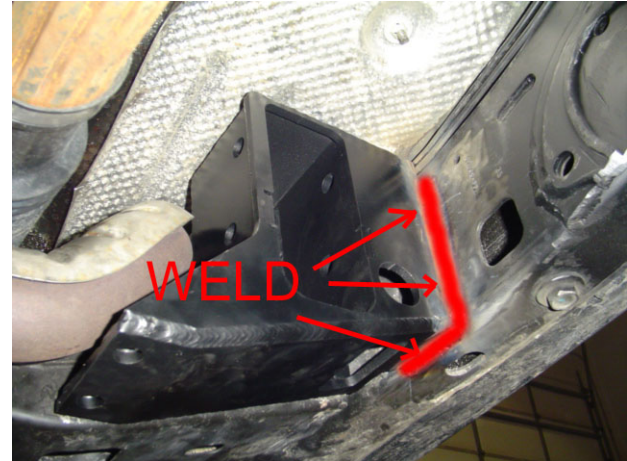
D.S. Bracket Welded in Place
