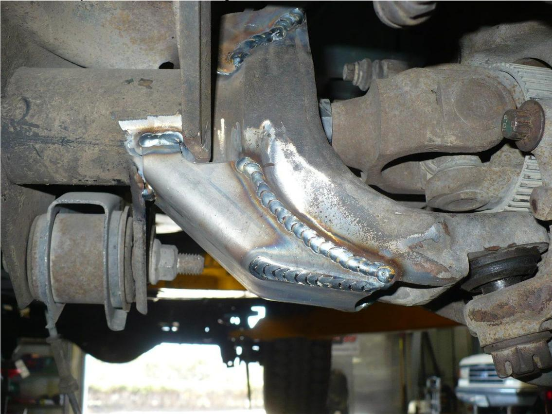
13) After welding, clean off any weld burrs and paint the desired color to prevent corrosion.
