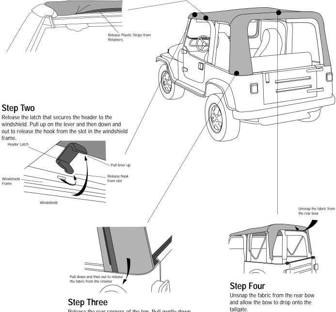
Release the rear corners of the top. Pull gently down and then out to release the plastic strip from the retainer on the vehicle.
