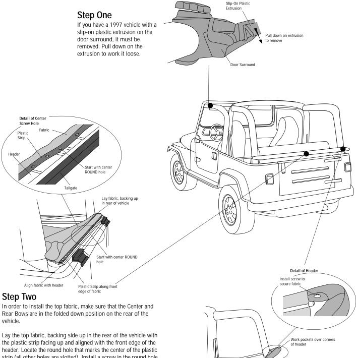
strip (all other holes are slotted). Install a screw in the round hole to secure the fabric to the header as well as to center the top. Then proceed to install screws in the remaining seven or thirteen holes along the front of the header.
