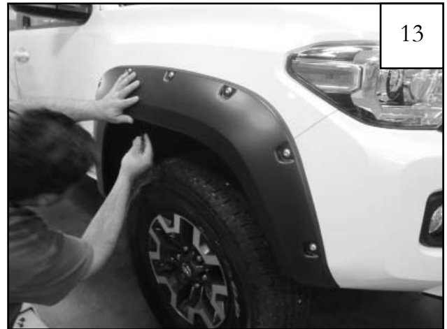
Position flare on fender, pressing inward on the flare, line up the flare mounting holes with the mounting clips on the bracket. Install 2 supplied screws (SW1-0036) through the flare and into the clips on the bracket. Do not tighten.
