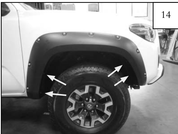
Still holding flare to fender, install supplied screws (SW1-0036) into remaining mounting holes (4 places).
