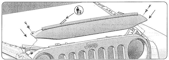
**4.** Position the light brow to the grill, hold the bottom away from face of grill until you get the mounting holes aligned. Once you are satisfied with the placement pull the red backer tape out across the top of the grill, once it is removed apply pressure across top of grill and to front of grill and reinstall the push plugs.
