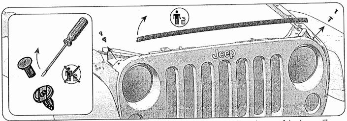
1. Using a straight blade screw driver, remove the two outer fasteners from the top of the Jeep grill. Do not discard, these will be reused. Remove the rubber gasket, some adhesive will remain on the grill, it is not necessary to remove all of the adhesive, discard the gasket.
