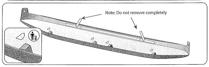
3. Remove the 4 pieces of red backer material from the adhesive tabs. Pull apx 3" of the red backer material away from the adhesive strip, do not remove completely. Position the backer material as shown in the drawing above.
