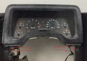
Remove the 4 screws securing the instrument cluster
