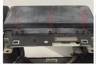
Remove and retain the front bezel screws located below the bezel in the lower right and left corners
