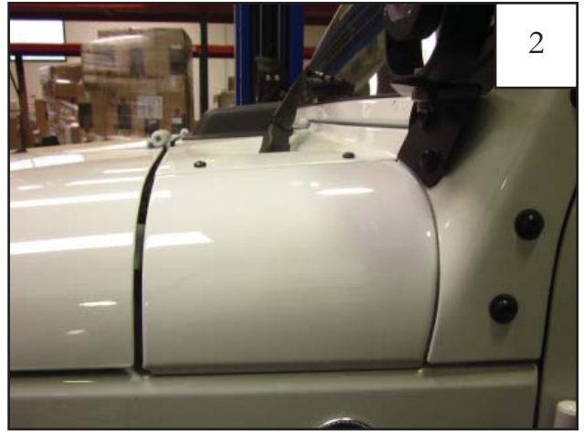
Using the supplied alcohol wipe, clean area where part will be placed. NOTE: Temperature should be between 60°F and 110°F for proper tape adhesion.
