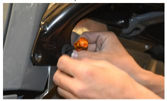
**32. Re-install any removed fasteners, then** go back over every bolt on the Crusher Flare and the JK Inner Fenders to ensure that each is tight. Push the LED lamp into place within its rubber grommet.
