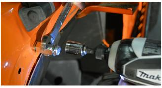
**25. Once the nut-sert has seated** correctly, loosen the bolt then remove it and the rest of the tool from the nut-sert. Install a new nut-sert onto the tool, oriented the same as the last, and set it aside until your next nut-sert installation. Inspect the nut-sert to make sure it is properly seated and that the surrounding sheet metal isn't excessively deformed. Note that some deformation of the sheet metal is normal, and that it will be covered by the part after installation.
