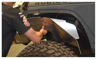
17. Hold the Inner Fender in place while re-installing the OE metric hex head bolts that were removed at the top of the wheel opening. They will pass through the two holes at the top of the Inner Fender, through the Crusher Flare Upper Sub-Frame Bracket, and into the threaded holes in the Jeep's sub-frame.
