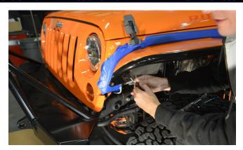
**14.** Unbolt and remove the Crusher Flare.
