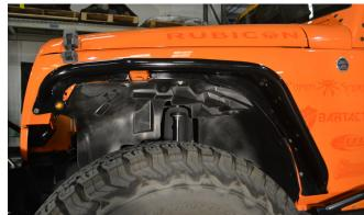
12. Optional: apply masking tape to the Jeep's fender, around where the flare attaches. This will protect the Jeep's paint finish in case the flare or the inner fender components are accidentally bumped against it during the following installation procedures.
