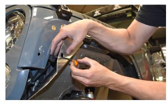
**31. Re-install the Crusher Flare while** feeding the 3/4" LED lamp through the corresponding light mount hole (it will be necessary to leave the rubber grommet disengaged from the barrel of the lamp.
