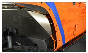
18. Re-install the Crusher Flare Lower Sub-Frame Bracket using ONE of the bolts that were removed, to attach it to the outer sheet metal of the Jeep's fender to hold it into place. Make sure the other hole in the bracket is aligned with the corresponding hole in the Jeep's fender.
