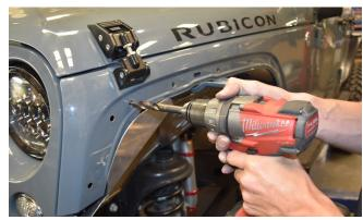
NOTE: It is HIGHLY RECOMMENDED to invest in a professional nut-sert installation tool, such as the Marson Giant Threadsetter, available from online tool sellers.
