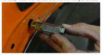
24. Use an open end wrench to hold the coupler nut stationary while turning the head of the bolt clockwise with a ratchet (or small impact wrench) and socket. As you turn the ratchet, the bolt will draw the far end of the nut-sert toward the inside of the sheet metal, gripping it with the knurled outside edge of the nut-sert as it deforms. Continue to turn the ratchet until the nut-sert is fully seated. DO NOT OVER-TIGHTEN as you can damage the nut-sert, or cause it to lose its grip.
