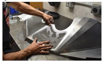
9. Use a hex key and ratchet with socket to tighten each of the screws/nuts to secure the Mesh Inserts into place. Tighten the fasteners in a criss-cross pattern, and check that the Mesh Insert is seating squarely against the Inner Fender without warping, as you tighten each fastener. Also continue to check that the Mesh Insert remains centered.
