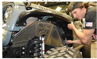
27. At the front-lower corner of the Inner Fender, find the screw-tab which should be resting against the Jeep's body tub sheet metal just above the forward body mount. It may need to be pushed slightly into place. Use the supplied self-tapping sheet metal screw to secure the Inner Fender to the body tub at this screw-tab location. The following photo depicts drilling a pilot hole
