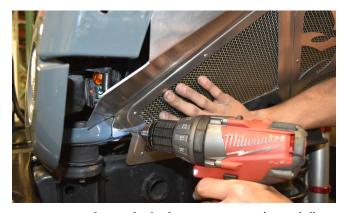
28. Use a rotor-broach, hole-saw or step-bit to drill out the 3/4" hole at the forward LED lamp location. If using a rotor-broach or hole-saw, it may be possible to use the hole in the Crusher Flare as the drill guide. If using a step-bit it will probably be necessary to temporarily remove the Crusher Flare after marking the hole location, but before drilling the hole.
