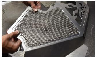
4. The supplied hardware is used to attach the Mesh Insert to the Inner Fender by passing the screw through the hole in the Inner Fender, then through one of the gaps in the mesh. What makes this slightly tricky is that the threads on the screw are slightly larger than the openings in the mesh, so a small Phillips screwdriver or similar tool must be used to slightly round-out the square opening in the mesh where the screw will pass through. DO NOT
