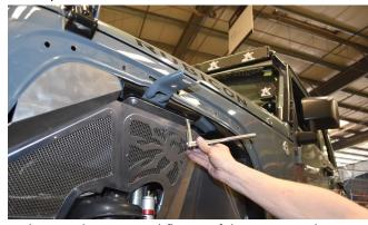
Make sure the rearward flange of the Inner Fender piece aligns correctly into the pocket where the Crusher Flare Lower Sub-Frame Bracket was removed, then tighten the two OE metric hex head bolts at the top of the Inner Fender.
