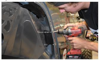
Once this hole has been drilled, remove the outer bolt from the other hole location, install the inner bolt at the new location using another of the supplied serrated flange nuts, leaving the Lower Sub-Frame Bracket installed with only the two inner bolts in place (the two bolts which pinch
