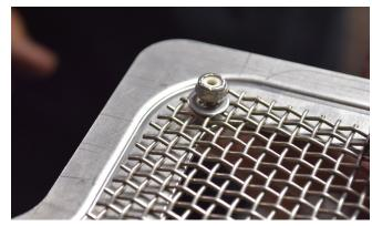
7. Continue with the rest of the fasteners on the same Mesh Insert. Work one fastener at a time, beginning with the adjacent fastener to the previous, and work in a circle until all fasteners are installed. Between each fastener, recheck that the Mesh Insert is still centered around the edges of the vent hole in the Inner Fender.
