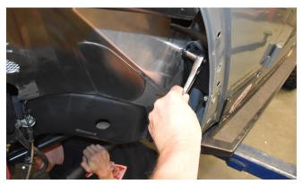
**22. One of the flare mounting** bolts is in a location that will be impossible to access the nut on the back side of the panel after the Inner Fenders have been installed. A 5/16-18 nut-sert will need to be installed in this difficult bolt hole location, which is directly below the hood latch on either side of the Jeep. Drill this hole out to 17/32" in preparation for installing one of the supplied 5/16-18 nut-serts.
