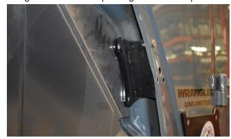
19. Use a 3/8" bit to drill through the second (un-bolted) hole in the Lower Sub-Frame Bracket, using it as a drill
