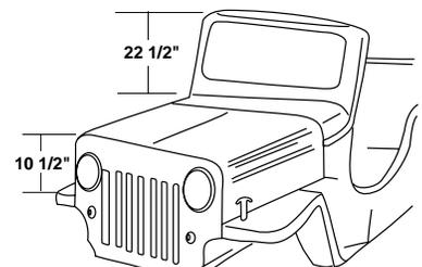
Windshields are sometimes interchanged on older model vehicles. The vehicle's windshield and body style are the key factors that determine which convertible top model number fits a particular vehicle. These diagrams will help you identify your vehicle to determine which top you need.
