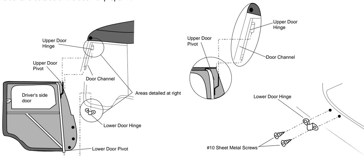
**Note:** After installation of the door, the frame of the door may be bent slightly to fit the contour of the vehicle body.
