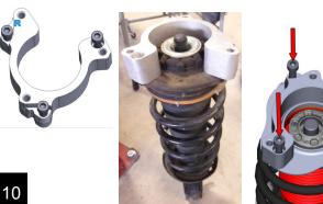
Re-install the strut using the factory bolts in the bolt holes of the spacer. The letter R will go toward the front of the Jeep. Do not apply loctite to these bolts. Torque to 50 ft-lbs.
