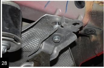
Remove the bolt supporting the brake/abs lines bracket. Insert provided 1.00" spacers and install M8 X 50mm bolt with washer. Apply blue loctite and use a 13mm to tighten.
