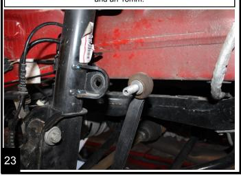
**Loosen** the unibody side lower control arm bolt with an E-20 Reverse Torx and a 17mm. Do not remove.
