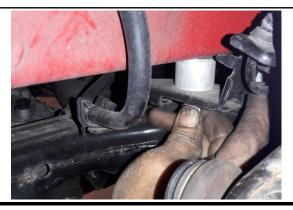
Support the lower sub-frame on a jack. Remove the 4 bolts with an E-20 Reverse Torx.
