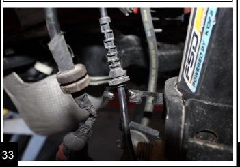
With an E-16 Reverse Torx and a 16mm, remove the 2 bolts that attach the knuckle to the strut.
