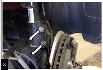
Remove the 3 upper strut bolts with an E-14 Reverse Torx and remove the strut.
