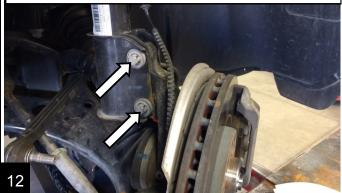
Insert the lower stud of the quick disconnect sway bar linkage into the factory sway bar. Place 7/16" washer and M12 nylock nut onto the stud. Use a 6mm allen to hold the stud, tighten down the nut with a 18mm wrench.
