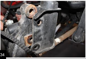
Remove the 3 upper bolts with an E-16 Reverse Torx and remove strut. Install spacer using 10M x 50mm Allen Bolts, *with blue loctite*, into recessed holes (no washers). With an 8mm allen **torque bolts to 70 ft-lbs**.
