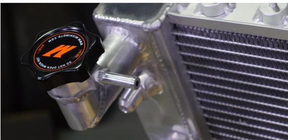
18. Snug the drain bolt on the Mishimoto radiator. (1x 19mm drain bolt)
