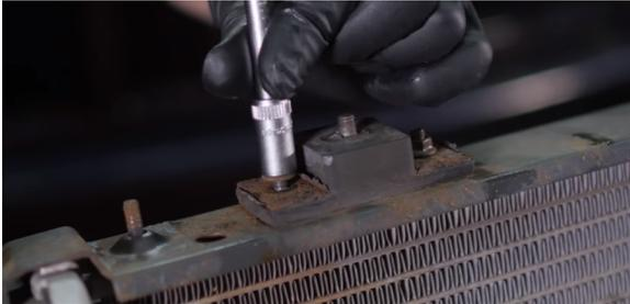
16. Locate the filler neck hardware included with your kit. If you have a newer style jeep or you are converting to an open cooling system, you will install the fitting with the overflow tube. If you have an older style jeep, you will install the plug.
