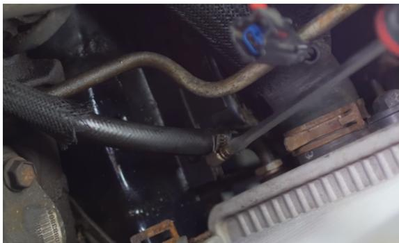
11. Loosen the flare nut that secures the upper
