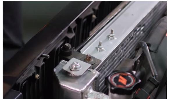
30. Install the upper isolators to the radiator and secure them with the provided hardware. (4x 10mm nuts)
