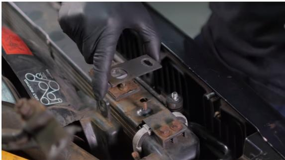
10. Place a drain bucket under the driver side of the radiator and loosen the clamp that secures the lower transmission cooler line to the fitting. Then remove the line from the fitting.
