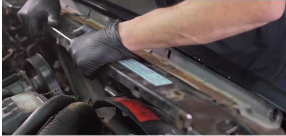
9. Remove the thread cutting nut, nut, and washers that secure the AC condenser bracket. Then remove the bracket. Repeat this process on the driver side.
