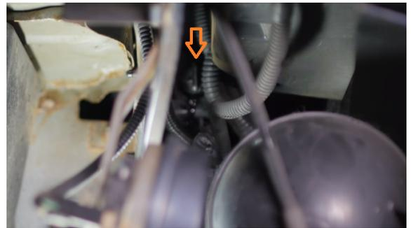
2. Remove the overflow hose from the radiator filler neck.
