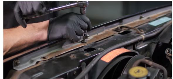
8. Remove the six bolts that secure the radiator support to the vehicle. Then remove the radiator support and trim panel from the vehicle. (6x 10mm bolts)
