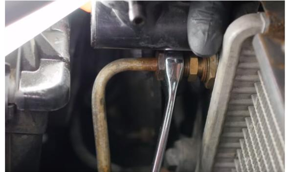
12. Compress the clamp that secures the lower radiator hose and separate the hose from the radiator. (1x spring clamp)
