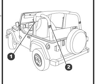
Use pliers to squeeze the top tabs, if necessary, to align the holes and improve ease of installation of the Bracket Bumpers.
