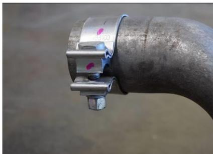
1. Be sure to check all parts are correct and match the Manual. Loosen the factory OEM clamp located just in front of the muffler above the factory axle. This will require a 15MM.
