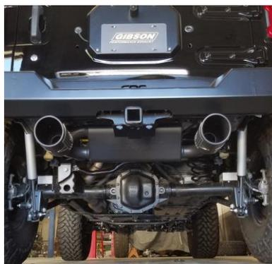
6. Slide the 2.5" band clamp over the expanded part of the muffler and make clamp snug but not tight. Install the Gibson provided tips. Check for exhaust clearance before tightening.
