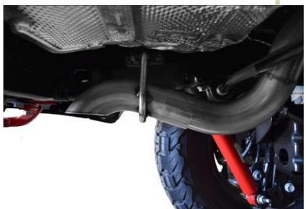
8. To install your XT Tip simply remove the exhaust from the Gibson head pipe and re install the tip using the same clamp and driver side only hanger. Protect your tips when in storage. We do not want any dings or dents.
