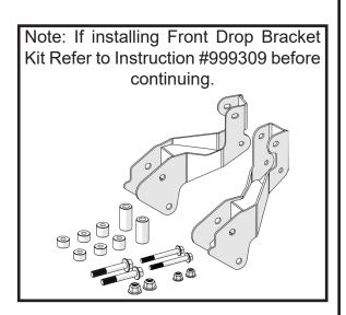
\*LEAVE CONTROL ARM BOLTS LOOSE UNTIL THE END OF THE LIFT INSTALLATION\*
