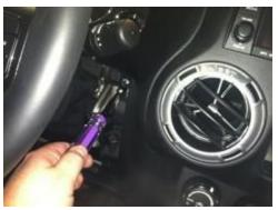
**Step 25:** Remove center stack/cluster surround. **Step 26:** Remove glove box for access and run Chassis Harness toward the center of the dash.
