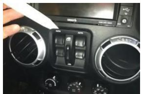
Step 21: Disconnect harness from window switches.
