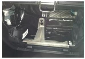
**Step 27:** Using a plastic trim removal tool, remove the HVAC panel.
