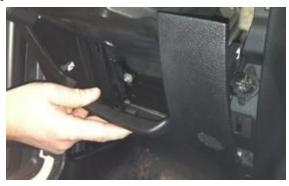
**Step 24:** Remove (2) 7mm bolts on both sides of the steering column.
