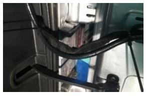
**Step 10:** Use a T20 Torx bit to remove the subwoofer box.( If equipped)
