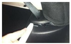
**Step 12:** Using a plastic trim removal tool, remove the rear access panel to expose 10mm bolt, and remove the bolt.
