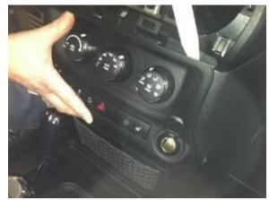
**Step 28:** Run Red 12v+ ignition wire of supplied Chassis Harness to the ignition controlled power point/cigarette lighter below HVAC panel.
