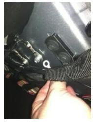
**Step 17:** In the factory wire harness located in the passenger's footwell, locate the White/Gray Reverse signal wire and splice Green Reverse wire from supplied Chassis Harness. RECOMMENDED: Use solder and cover with heat shrink tubing or use T-tabs as an alternate connection method.
