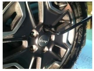
**Step 2:** Slide Camera on studs placing harness end inside of tire carrier. *Do not run harness through the camera bracket opening*.
