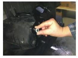
**Step 5:** Plug the Camera connector into the gray Chassis Harness connector, and insert RCA connector end of supplied Chassis Harness through the rear gate vent behind tire carrier.
