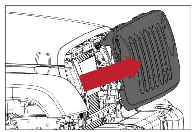
3. Remove factory headlight bolts. Then use supplied M6 Button Head Bolts to attach Elite Headlight Gaurd. Next, reinstall grille, see steps 1 and 2.
