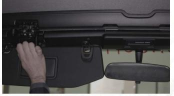
2. LOCATE TORX SCREWS. Remove the two T-25 Torx Screws on top of the roll cage.
