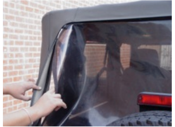
2. Unzip rear window and remove.
